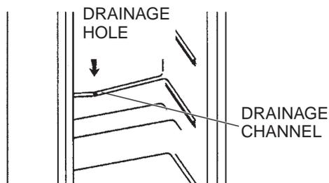
avoid the build up of impurities. Wipe the channel with a damp cloth and use the cleaning tip to clean out any residue from the drainage hole.
