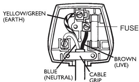
The wire which is coloured BROWN must be connected to the terminal which is marked with the letter L or coloured RED or BROWN.
